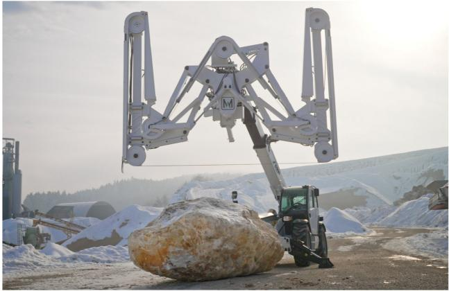
Schwing GmbH has developed a mobile diamond wire saw (MDS) for various quarry requirements. It is compact, can be moved quickly and does not need to be installed stationary. The design is already in use at the Bamberg natural stone plant, among others, and will be presented at Marmomac 2023.
