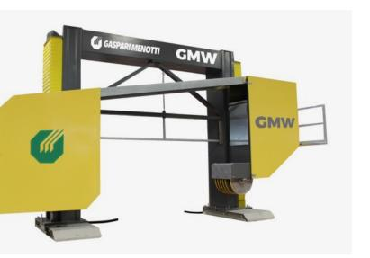
It is the most flexible among the GMW Series multiwire machines, which keeps intact the philosophy of reliability and robustness typical of Gaspari Menotti brand. SMARTWIRE GMW 06 multiwire machine has been designed to allow to simultaneously cut up to 5 slabs of different thicknesses in a simple and precise way.
