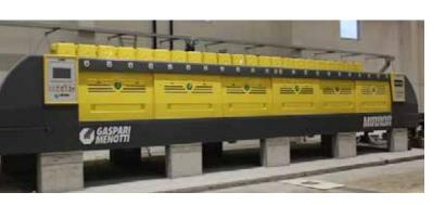
Mirror slabs polishing machine, available in marble, granite and quartz versions, represents the vanguard in its category thanks to a solid and compact structure. The machine was designed to ensure very high productivity and quality of the finished slabs, thanks to mechanical solutions - beam speed up to 75 m / min - and electronic - sensors that adopt IO-LINK standards - offering top-level performances even on difficult materials. In particular, the IO-Link
