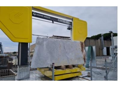
Our single wire machine is the right solution for squaring marble and granite blocks and for cutting thicknesses. The wire is rotated by means of four large flywheels, each with a diameter of 1200mm, one of which is motorized.
